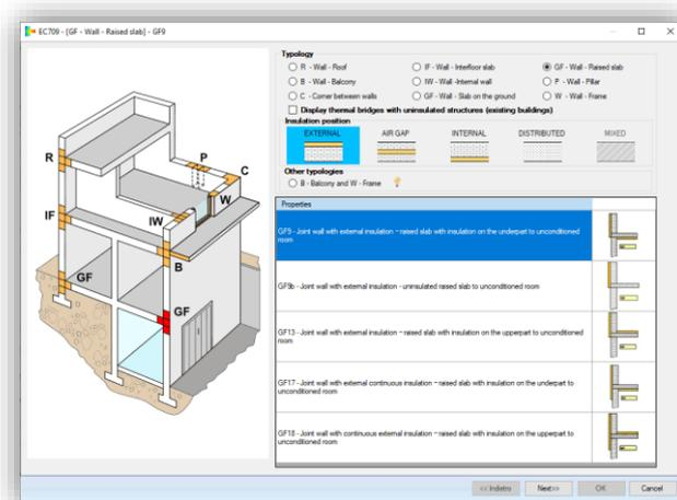
Once the type of thermal bridges have been chosen, it is possible to proceed to its characterisation, which involves specifying the **main characteristics** of the structures that compose it (thermal transmittances, thicknesses, conductivity of bricks, etc.), thus determining precise linear thermal transmittance values.
