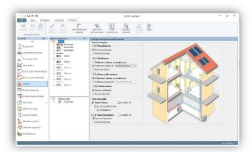
The software allows the simulation of the presence in the building of systems for **transporting people or goods** (e.g. lifts), in accordance with **UNI/TS 11300-6**, as well as the determination of the energy requirements for **artificial lighting** in buildings for non-residential use (indoor rooms, outdoor areas, absorption of parasitic electrical energy due to control and emergency systems), in accordance with **UNI EN 15193.**
